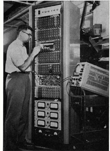
**THE "SCRAMBLER,"** electronic coder that scrambles signals, is assembled at the Skiatron laboratories. The decoder (below) unscrambles picture when subscriber inserts card and presses a button. Card also records programs viewed for billing purposes.
